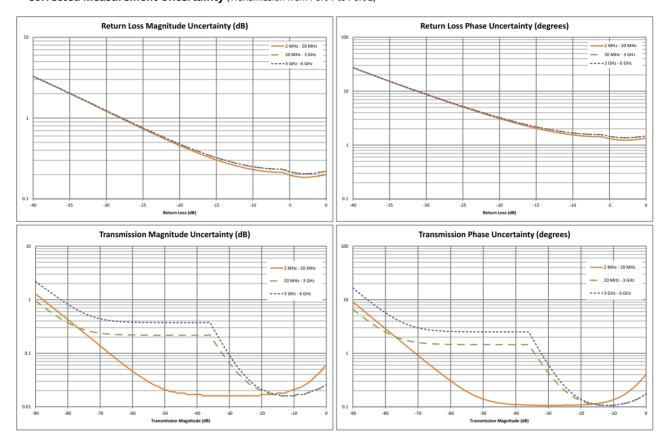
Full 1-path, 2-port forward path calibration with isolation, high power, 10 Hz IFBW, no averaging, 10 minute warm-up. OSLN50A-8, OSLNF50A-8, TOSLN50A-8, or TOSLNF50A-8 calibration kit. Reflection and Transmission Tracking are typical.
